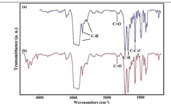
Figure 11. FT-IR spectra of PA-2 sample (a), before and (b) after oven aging at 100°C for 60 days.
