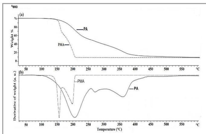
Figure 7. (a) TGA and (b) DTG curves of PA and PMA.
