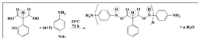
Figure 4. The step-growth polymerization of PMA and PD.
