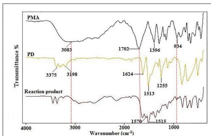
Figure 3. FT-IR spectra of PMA, PD and the reaction product.
