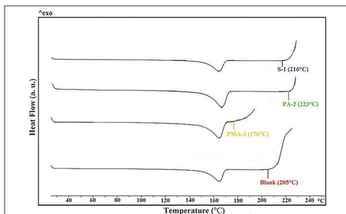
Figure 8. DSC curves of the PP samples obtained from OOT test.
