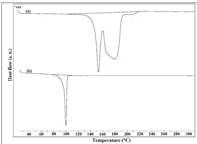
Figure 5. DSC curves related to purified a) PMA and b) PA.
