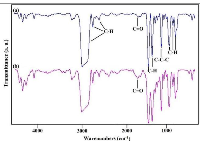
Figure 10. FT-IR spectra of Blank sample (a), before and (b) after oven aging at 100°C for 60 days.
