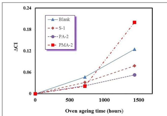
**Figure 12.** Change of carbonyl index ( $\Delta CI$ ) for the film samples as a function of time of oven aging at 100°C.
