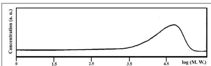
Figure 6. Gel permeation chromatogram of PA.
