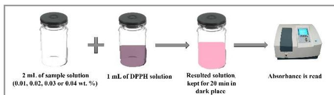
**Figure 2.** Schematic representation of antioxidant capacity determination by free radical scavenging.
